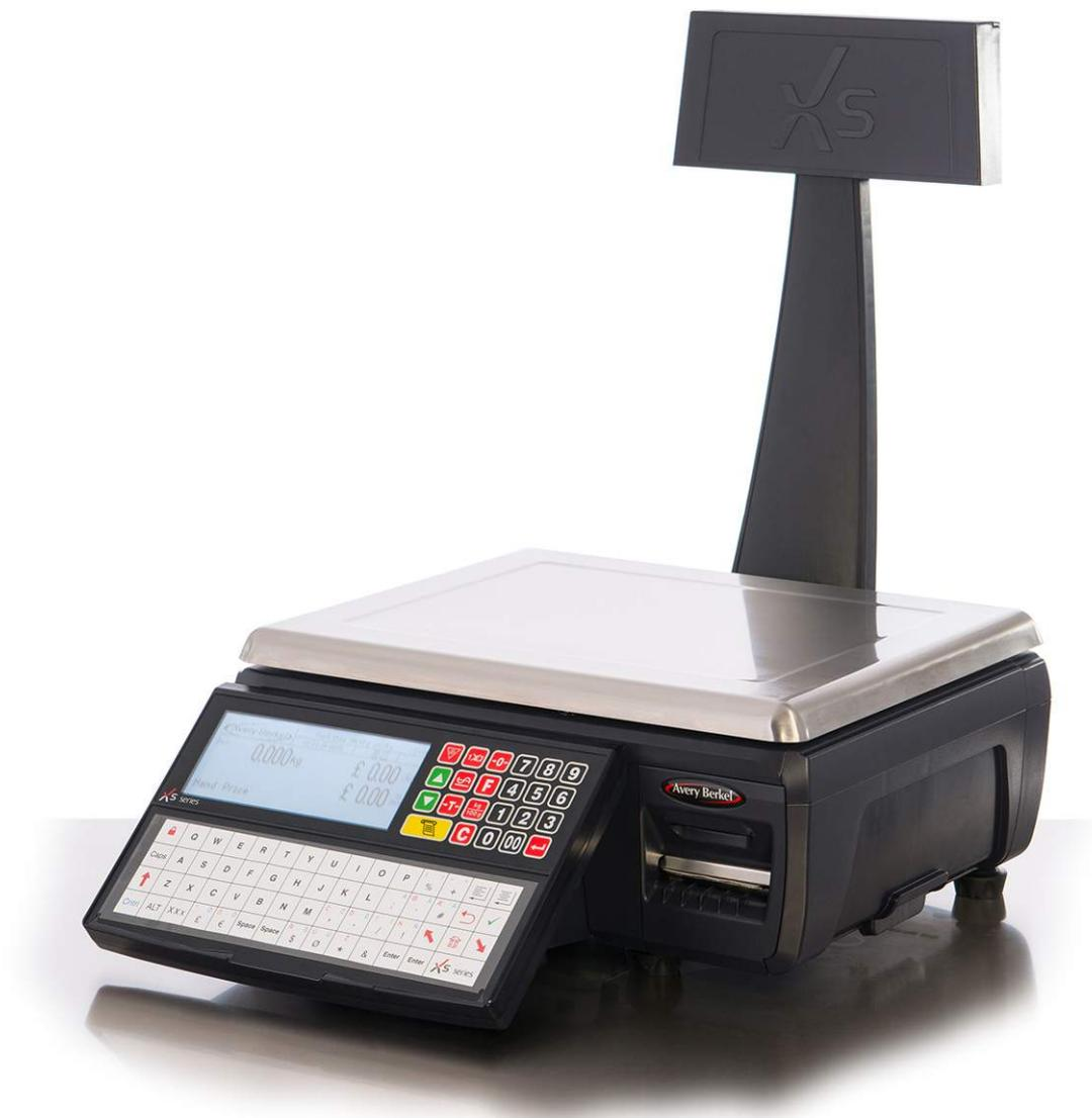
Scale with column mounted customer display and a vendor display located on the base unit. The display, keyboard and weighing characteristics are identical to the mono bloc unit. The scale has a 58 pre-set key keyboard for PLU selection and an additional 23 full-travel tactile keys for regularly used functions.
